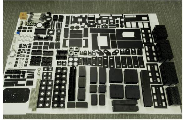
Fig. 4. The structural components for a single THOR-OP robot use standardized dimensions.
