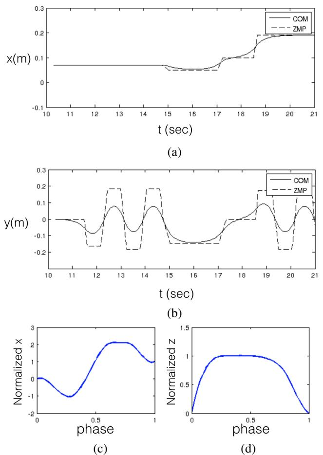
Fig. 6. COM, ZMP and foot trajectories during strong kick motion. (a) X axis COM and ZMP trajectories (b) Y axis COM and ZMP trajectories (c) X axis foot trajectory during kick step (d) Z axis foot trajectory during kick step
