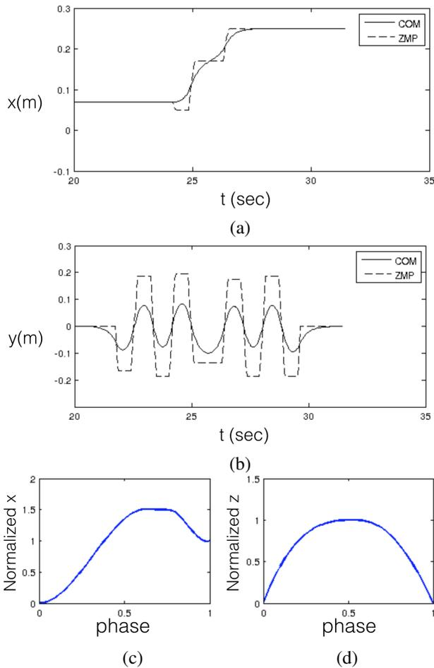
Fig. 5. COM, ZMP and foot trajectories during fast kick motion. (a) X axis COM and ZMP trajectories (b) Y axis COM and ZMP trajectories (c) X axis foot trajectory during kick step (d) Z axis foot trajectory during kick step
