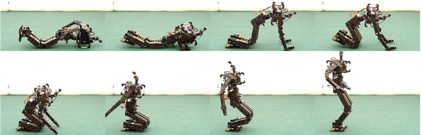
Fig. 2. THOR-OP robot performing getup motion from the prone posture
