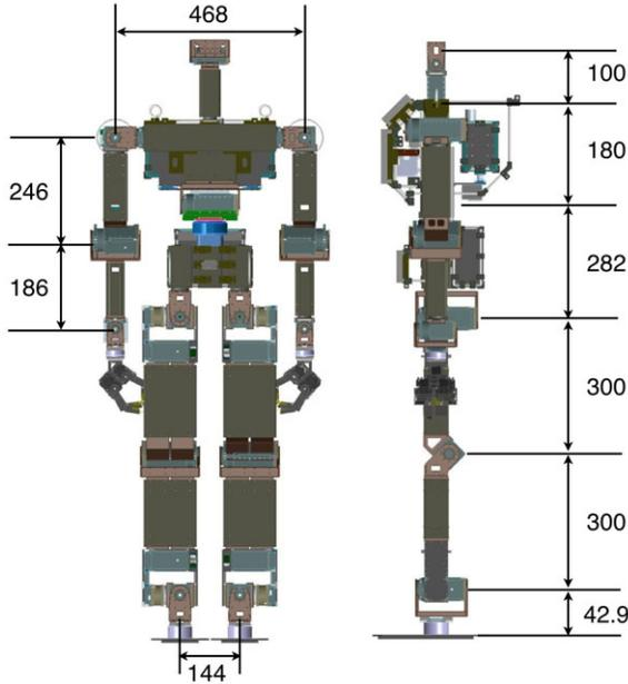
Fig. 3. Front and side views of the THOR-OP robot with dimensions. (unit: *mm*)
