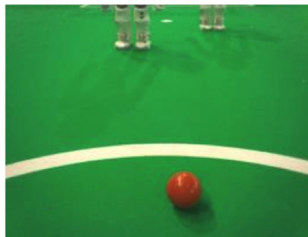
Fig. 1. A typical image used to learn the color of the surface of play, the color of line markings and the color of the ball.
