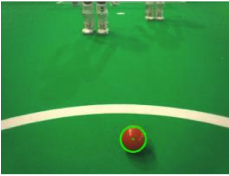
Fig. 2. A typical result of the Hough transform for finding circles of size similar to an expected nearby ball.
