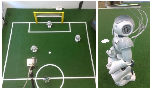
Fig. 4. The general setup of the experiments. Three robots are on fixed positions on the field. The observing robot is provided with ground truth pose information from the SSL-Vision system. For this purpose, it has a pattern attached to its head that is tracked by a camera.
