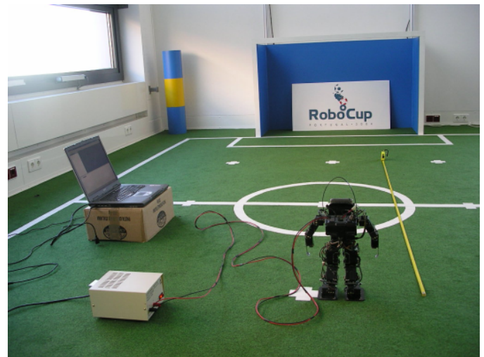
Fig. 7. The optimization scenario for the real robot on a RoboCup Humanoid Kid-Size League field
