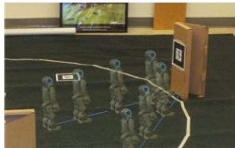
Fig. 4: Landmark detection experiment design from an aerial perspective. The rectangle represents the landmark and the circle represent the different robot positions.
