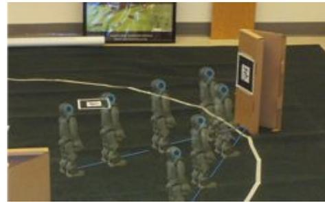
Fig. 4: Landmark detection experiment design from an aerial perspective. The rectangle represents the landmark and the circle represent the different robot positions.
