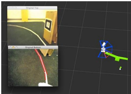
Fig. 3: The *rviz* visualization of the affordance calculation. The robot model is shown in white. Blue triangles represent navigable affordances and red triangles non-navigable ones. The green lines show all the lines taken into account in the affordance calculations. The output of both cameras is also shown in the left margin and the output of the Hough algorithm is shown for the bottom camera.
