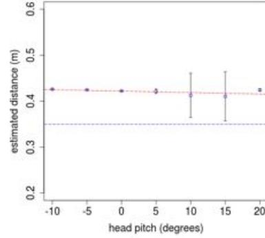
Fig. 7: The estimated distance to the line as a function of the ground truth for the head pitch angle experiment. The blue line represents the constant function at the real distance (expected behavior). The red line shows a least squares regression of the data. The angle values correspond to those accepted by the *NAO* API.
