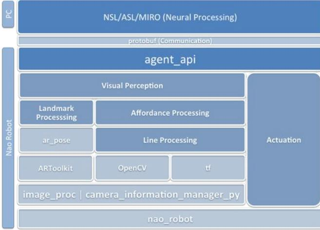
Fig. 2: Architecture diagram. Light shaded rectangles represent third party packages whereas the dark shaded ones are developed in this work.
