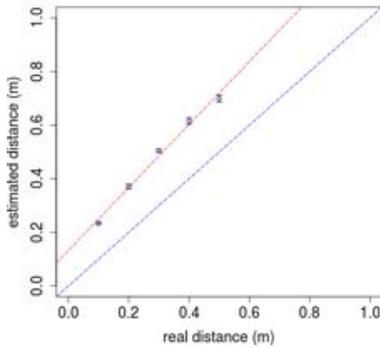
Fig. 6: The estimated distance to the line as a function of the ground truth for positions in the 45 degree skew line with respect to the landmark. The blue line represents the identity function (expected behavior). The red line shows a least squares regression of the data.
