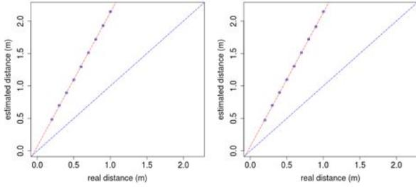
Fig. 5: The estimated distance to the landmark as a function of the ground truth for positions in the perpendicular line (left) and in the skewed line (right) with respect to the landmark. The blue line represents the identity function (expected behavior). The red line shows a least squares regression of the data.
