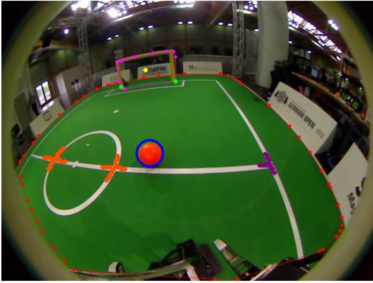
Fig. 6. A snapshot from the NimbRo-OP camera showing the detected features and the distortion induced by the fisheye lens.
