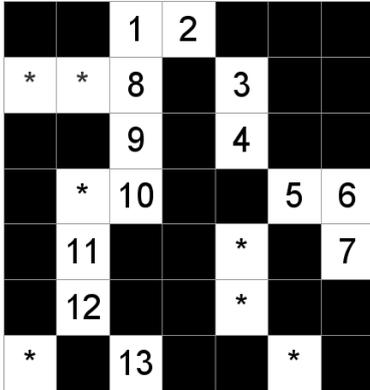
Fig. 4. An example of the chaining of the connected edges. The numbers show the insertion order. Pixels marked with an asterisk are not inserted in the current chain, even though they are connected to the others.
