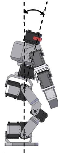
Fig. 3 The tilt inclines the centre of gravity to balance the robot.
