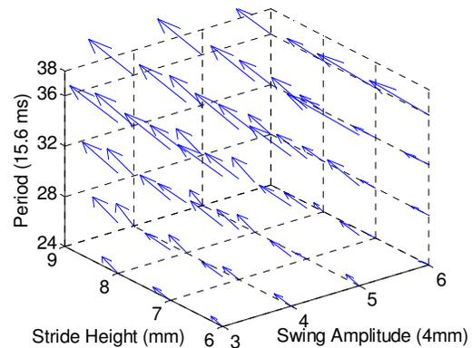
Fig. 13 3D parameters space and results. For each of the three variables four different values were tested resulting in  $4^3$  or 64 measurements. At each point in parameter space, a vector is drawn with the lateral head displacement as the horizontal component and the foot clearance as the vertical component. An ideal parameter set would result in a vector pointing vertically up.
