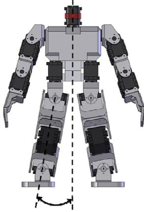
Fig. 5 Camber introduces a rotational offset on the hip and ankle joints to increase lateral stability and prevent collisions between servo skeleton elements.
