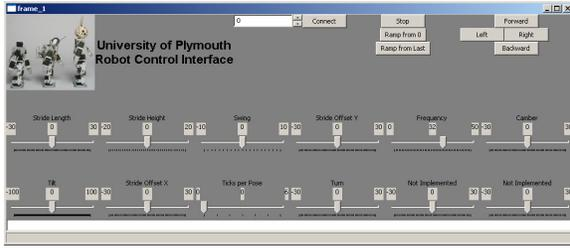
Fig. 10 PC based interface allows rapid adjustment of Gait Parameters.
