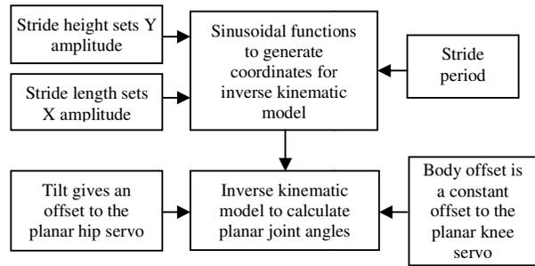
Fig. 8 Overview of robot kinematics of the hip, knee and foot servos with parallel axis.
