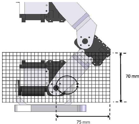
Fig. 2 The joint angles for each of the grid points are pre-computed and stored in the onboard microprocessor. The curve indicates the trajectory of the foot defined by (1) & (2).
