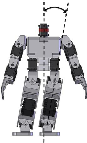
Fig. 6 Swing Amplitude controls how far the centre of mass of the robot shifts.
