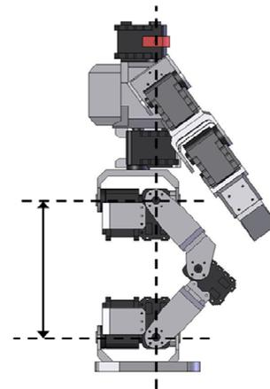
Fig. 4 The body offset shifts the vertical origin of the coordinate system through which the foot moves.
