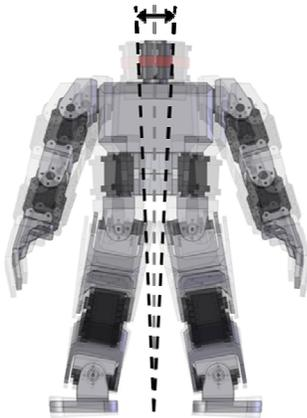
Fig. 11 Head displacement was measured as indicated.
