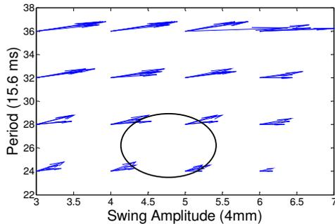
Fig. 14 Measured Quantities as a function of Period and Hip Swing amplitude. The multiple vectors at each point correspond to each of the measured stride heights.
