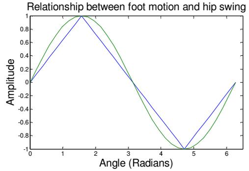
Fig. 7 The relationship between the swing of the hips (straight line) and the motion of the feet (curved line).
