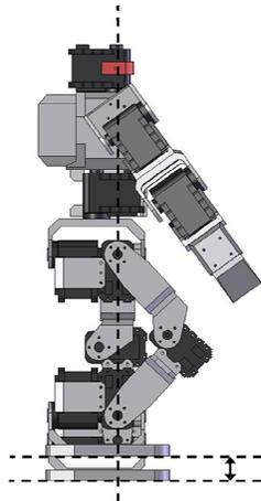
Fig. 12 Foot clearance quality was based on the foot completely leaving the surface.
