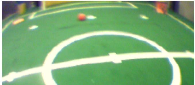
Fig. 7. Real-time experiment: The robot is supposed to approach the ball (middle). Other orange objects – a felt cloth (left) and a book (right) – are placed on the field in order to distract the robot.
